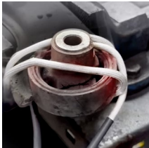
Extraction of a mounting bush
