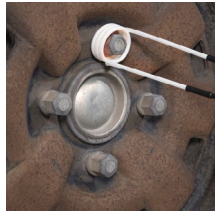
Loosening seized wheel nuts
