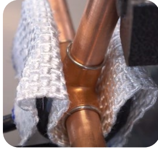
Assembly of copper parts with rings
