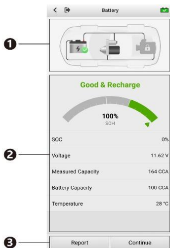
Figure 4-6 Sample Battery Test Result Screen
