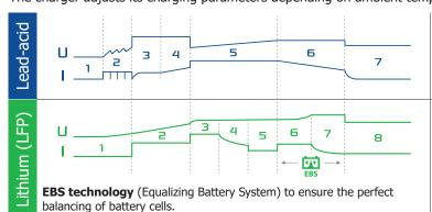
Specific 7 step charging curve for each battery technology. Can be safely left connected without supervision.
